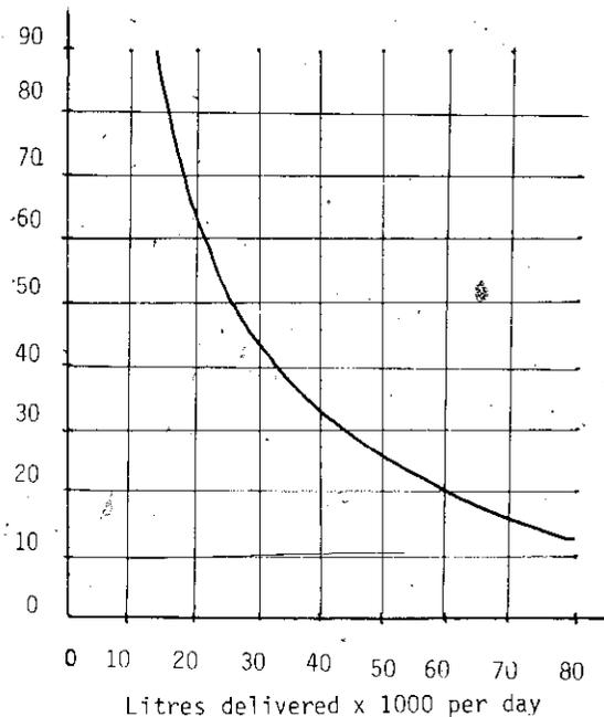
Recommended (Galvanized Iron) Drive Pipe: 50mm diameter, 18.5m length. Recommended (Plastic) Delivery Pipe: 25mm diameter. Minimum water supply required, 90 litres per minute. Ratio of waste water to delivered water = 6.56/1 @ 77m Delivery Head. Kinetic Energy conversion efficiency = 15.24% (Atmospheric vent). Optimum pump operational speed = 60 strokes per minute.
