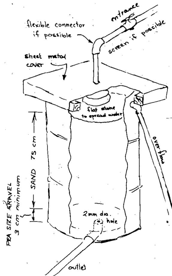
will be washed away. Fix the water intake so that there is always a small overflow. Screen the intake and provide a settling basin to help keep pipes from becoming plugged.
