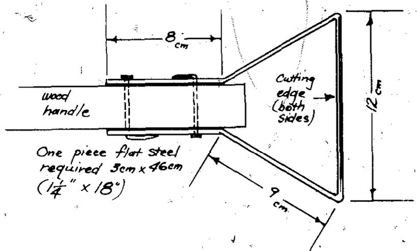
Mild steel works, since the triangular shape gives the weeder rigidity.
