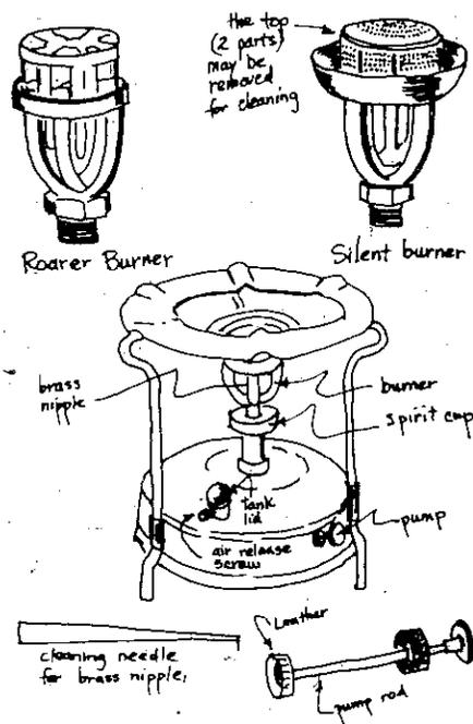
2. Fill the spirit cup with spirit and light the spirit. Care should be taken that the flame is out of the wind.
