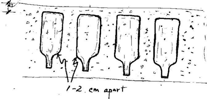
3. In pouring a concrete floor, you can place bottles neck down with a 1-2 cm space between each bottle and 1cm layer of cement on the top.
