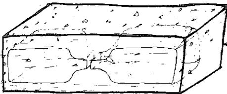
1. In building solid concrete blocks, two empty bottles in the centre of the block will save 15% in materials.
