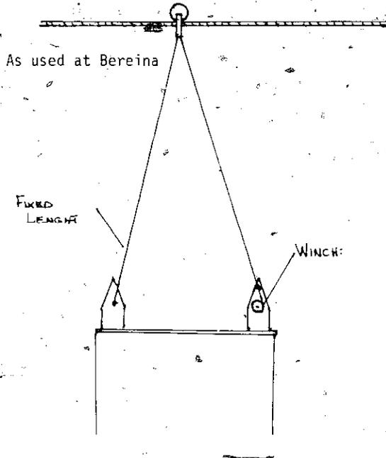
An alternative design: Use two tow cables, one with a fixed length, and one with a winch. To change direction or speed of travel, shorten or lengthen the second tow cable by using the winch.
