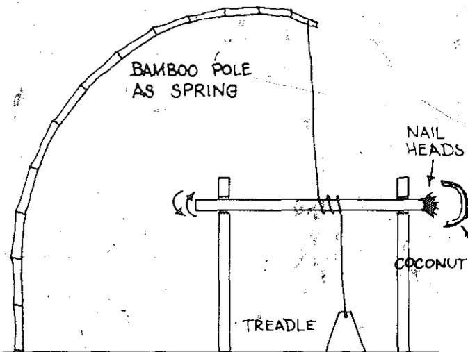
This is a simple treadle-operated scraper for extracting coconut, common in some parts of Indonesia, unknown in others. This appeared in *Appropriate Technology*, August 1975, where it was reported that the scraper was used successfully by BUTSI, the Indonesian Board for Volunteer Service, through a newly created village Technology unit. For more information on BUTSI write: Dr. W.P. Napitupulu, BUTSI Secretary, Tromol Pos 3290, Jakarta, Indonesia.
