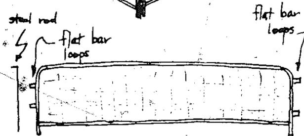
Panels made of pipes and hog wire. Use 3 or more.
