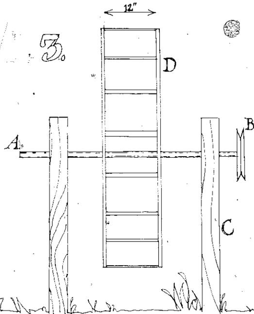
Figure 1: shows glued ply wood cleats fixing together wheel frames of 3" x 1" dressed hardwood used throughout.
