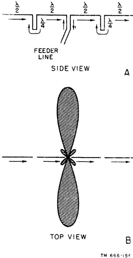
Figure 152. Typical collinear array.
