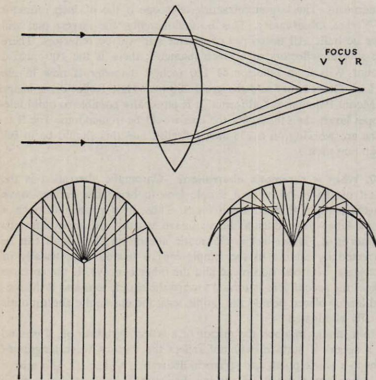
Single lens brings waves of light of different lengths to focus at different points. Correcting lens is needed to bring all wave lengths to focus at one point.
