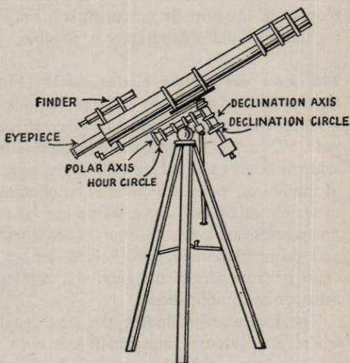
these is the polar axis, which is adjustable and is pointed precisely at the north celestial pole. The angle of the polar axis to the horizon, then, must be the same as the latitude of the telescope. There is usually a graduated circle, marked off in hours and minutes, attached to the polar axis. This is an hour circle and the figures on it correspond to the co-ordinates of right ascension of celestial objects. The polar axis must be capable of rotation.
