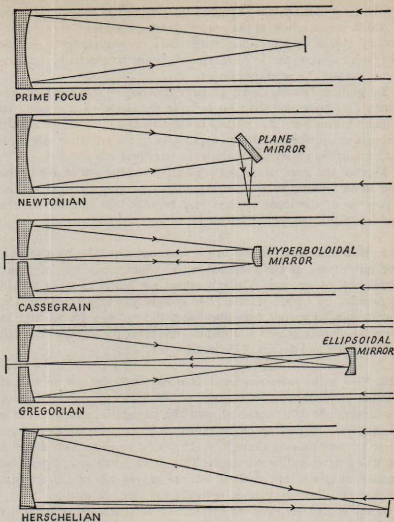
Optical systems of reflecting telescopes
