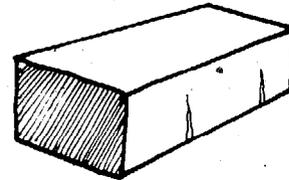
(b) Multiple surface cracks running in random directions are normally the result of differential drying shrinkage caused by the presence of lumps of drier material in the clay which do not shrink as much as the surrounding material. This fault arises from insufficient mixing of the clay before moulding or extrusion. Pebbles in the clay will have a similar effect and all of these faults will result in bricks with unsatisfactory shear strength.
