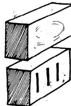
(e) Another kind of lamination crack can occur with bricks made by the sandmoulding process. This is caused when a piece of clay with sand covering its surface is inadvertently mixed into the clay of the brick. The film of sand separates the clay on either side of it so the brick will tend to split at this point if any stresses occur during drying or firing. The fault can also occur with oil moulding. Avoiding laminations from mould release substances is a matter of training.
