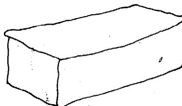
**Flashing on sides of top face** – this fault occurs with the use of fixed bottom moulds usually in production of frogged bricks. The spaces left down the sides to allow air to enter the bottom of the mould are sometimes wide enough for clay to protrude. This defect has been eliminated with the development of the hinged-bottom mould but these are not yet in widespread use.
