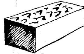
**Barmarks** – on the face of bricks can occur during the firing process with many types of raw material. If the preferred colour appears on the part of the face of the brick which is exposed to the kiln gases the remedy is to **flat set** the bricks so that all the stretcher faces are exposed. If on the other hand, the colour desired occurs only on the covered surface of the brick, they should be set face to face so that each brick has at least one stretcher face fully covered by another brick.
