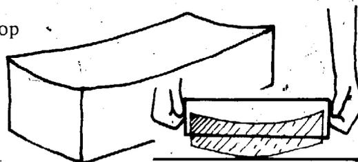
**Lip on bed face** – this is another moulding fault caused by the moulder not striking off the excess clay cleanly enough and leaving a 'flashing' around the edge.
