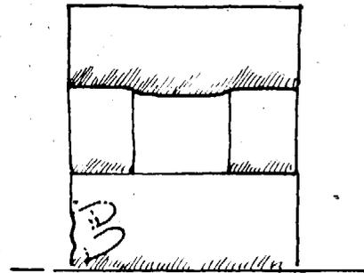
**'Banana shapes'** – differential rates of drying from one side to the other often distort the brick shape to the extent that it actually curves. This defect often rectifies itself automatically when the drying spreads across the brick, but if the top part of the brick becomes fully 'green hard' before the bottom has shrunk, the distorted shape remains. This problem can be avoided by gently turning over the bricks during the initial drying phase before the top side has dried completely hard.
