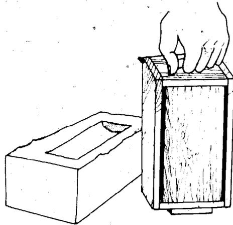
**Distorted or contaminated under-surface** – one of the main causes of imperfections to the brick shape is the drying floor not being smooth or covered with clean sand. The irregularities of the floor are transferred to the brick and any loose lumps of clay or pebbles in the sand become attached to the brick. These faults occur mainly when the bricks are set down flat with the slop moulding method.
