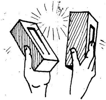
**Visible cracking** – also usually indicates that the brick is weak and may even fall apart during handling. Cracks can occur for a variety of reasons:
