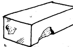
**'Dog-eared' corners** – are a common fault with extruded bricks and are caused by poor lubrication of the clay column as it emerges from the auger barrel. The defect occurs even with a well lubricated column if the raw material is too coarsely graded or badly mixed.
