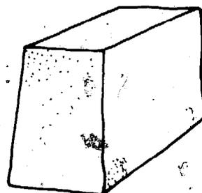
**Rounded corners** – the usual cause of a missing corner is a mistake by the moulder who failed to press enough clay into the mould box to fill it completely. Brick corners are also lost during rough handling while they are in the dry state and are particularly brittle.
