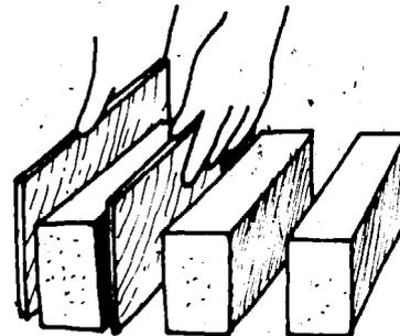
Oversize in **thickness** only. This fault frequently occurs with extruded wirecut bricks. In the cutting process a long length of extruded clay is forced sideways through a row of wires. These are frequently set at incorrect intervals leading to irregularities in the thickness dimension. If the other two green-size dimensions are too large, this should be a result of wear in the extrusion die and will be accompanied by some distortion of the rectangular cross-section.
