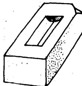
**Raised corners** – this is a common defect in slop moulded bricks caused by the corners of the brick sticking in the mould during the release movement.
