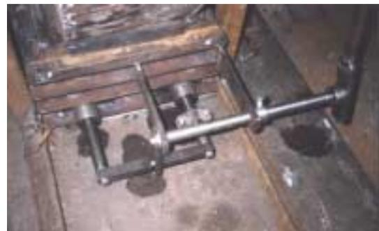
Ejection mechanism added
