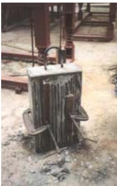
New cast concrete impactor
