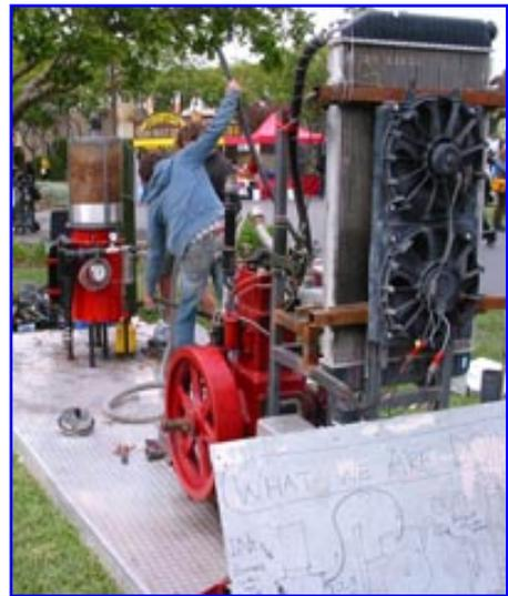
In addition to preheating the air, the heat exchange tubes also cool the product gas. I was surprised to see gas exiting the top of the gas cowl at 150-210F. Yes that is correct, 100C or less. Compare with typical no air preheating or gas cooling configurations which have gas exit temps in the 200-400C range. Hot gas is much more difficult to process downstream than cool gas. Cyclones, filters, plumbing and pumps are all complicated by high temp gas.
