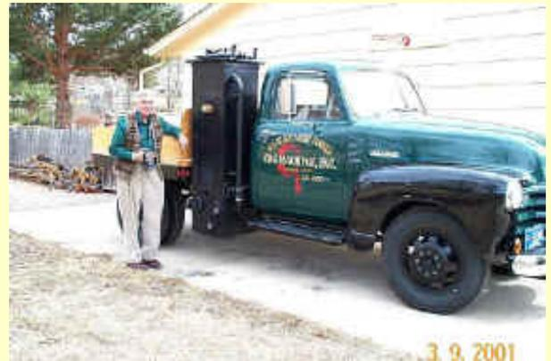
Mel turned on the auxiliary starting fan, and started the gasifier on large aspen chunks with a newspaper. After a few minutes he lit the gas at the front of the truck and started the engine. We drove around Colorado Springs for several hours. I realized what an art it was to drive a gasifier car, since he could control the spark advance, air fuel ratio and throttle, all from the steering column, while talking about the old and new days.
