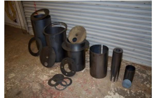
All Vessel Tubes, Flanges and End Plates
