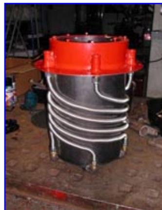
The internal geometry for this run was the "textbook" dimensions for Swedish inverted V hearth designs for a 2.5" reduction constriction. This is a very small constriction, intended for engines around 5-10hp. I did not do any special nozzle burn path tests or other diagnostic configurations, so i'm sure what I had could be improved upon. The fuel was walnut shells in 1/4 - 1/2 shell form. Moisture was measured at 15%.
