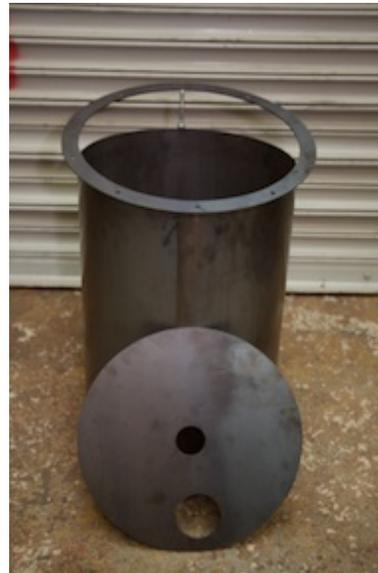
Gas Cowling Tube, Flange, and End Plate
