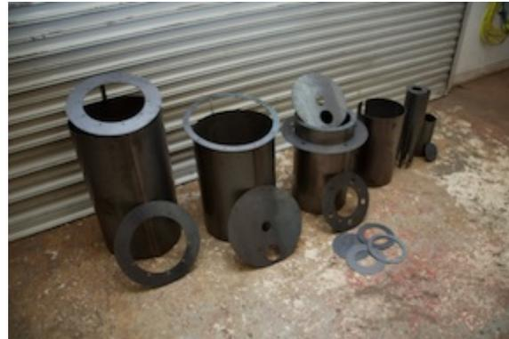
All Vessel Tubes, Flanges and End Plates
