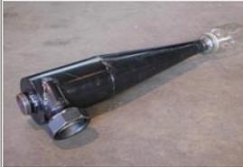
This is the standard 5" diameter cyclone from the GEK kit. It comes with a 2" box flange attachment at the inlet, and a 2" threaded NPT nipple for the outlet. A glass Mason jar and adapter is included for the particulate/condensate/tar catch.
