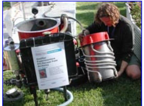
The above pictures show a new air preheating scenario for the GEK nozzle and constriction (Imbert) type downdraft reactor. We ran this configuration at the Maker's Faire in San Mateo, CA, May 4-5 to drive a Lister 6/1 diesel genset in dual fuel mode. The
