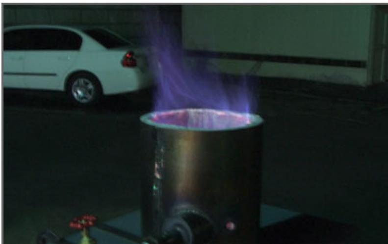
Clean hydrogen flame, invisible during daylight.
