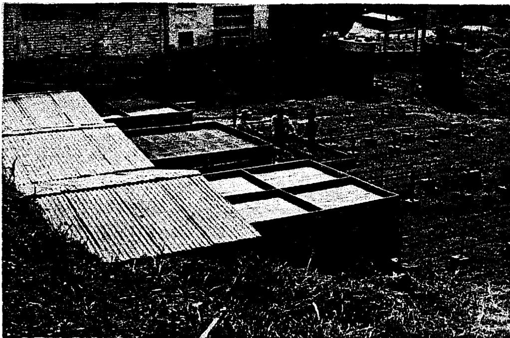
Figure 2a - Coffee drying carts. Each tray has a drying surface of 10 m<sup>2</sup>
