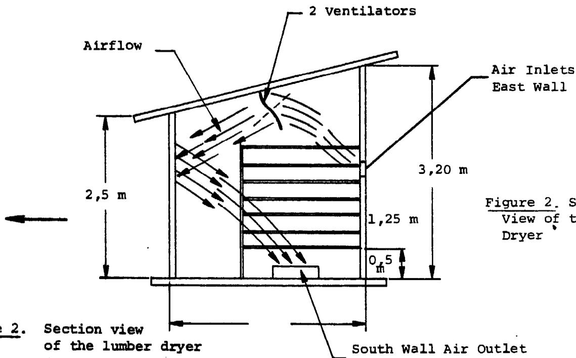
Figure 2. Section view of the lumber dryer
