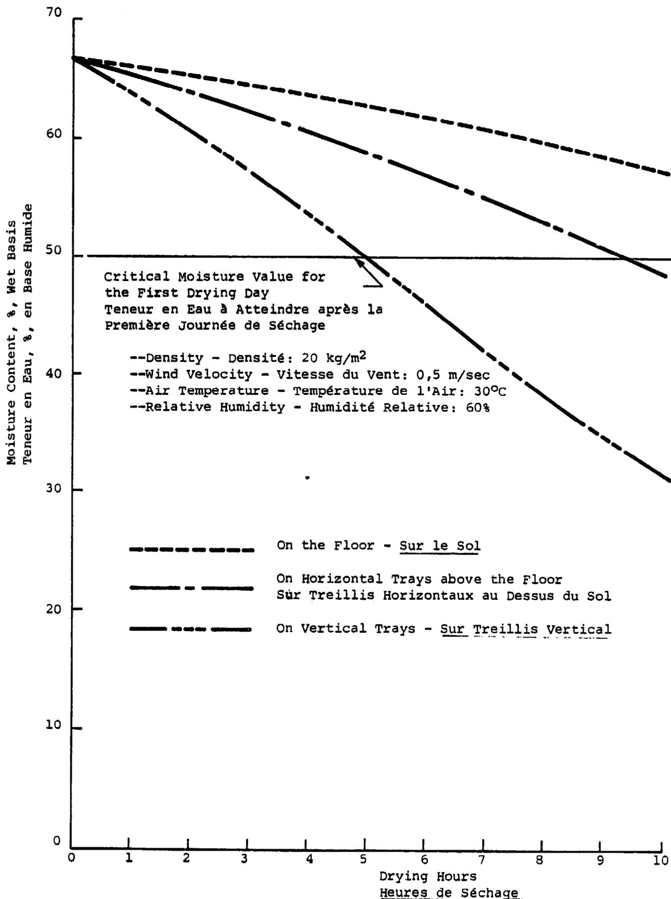
**Figure 5.** Drying Curves as a Function of Different Drying Systems Using Bars 0,9 x 0,9 x 5,0 cm (Simulated)
