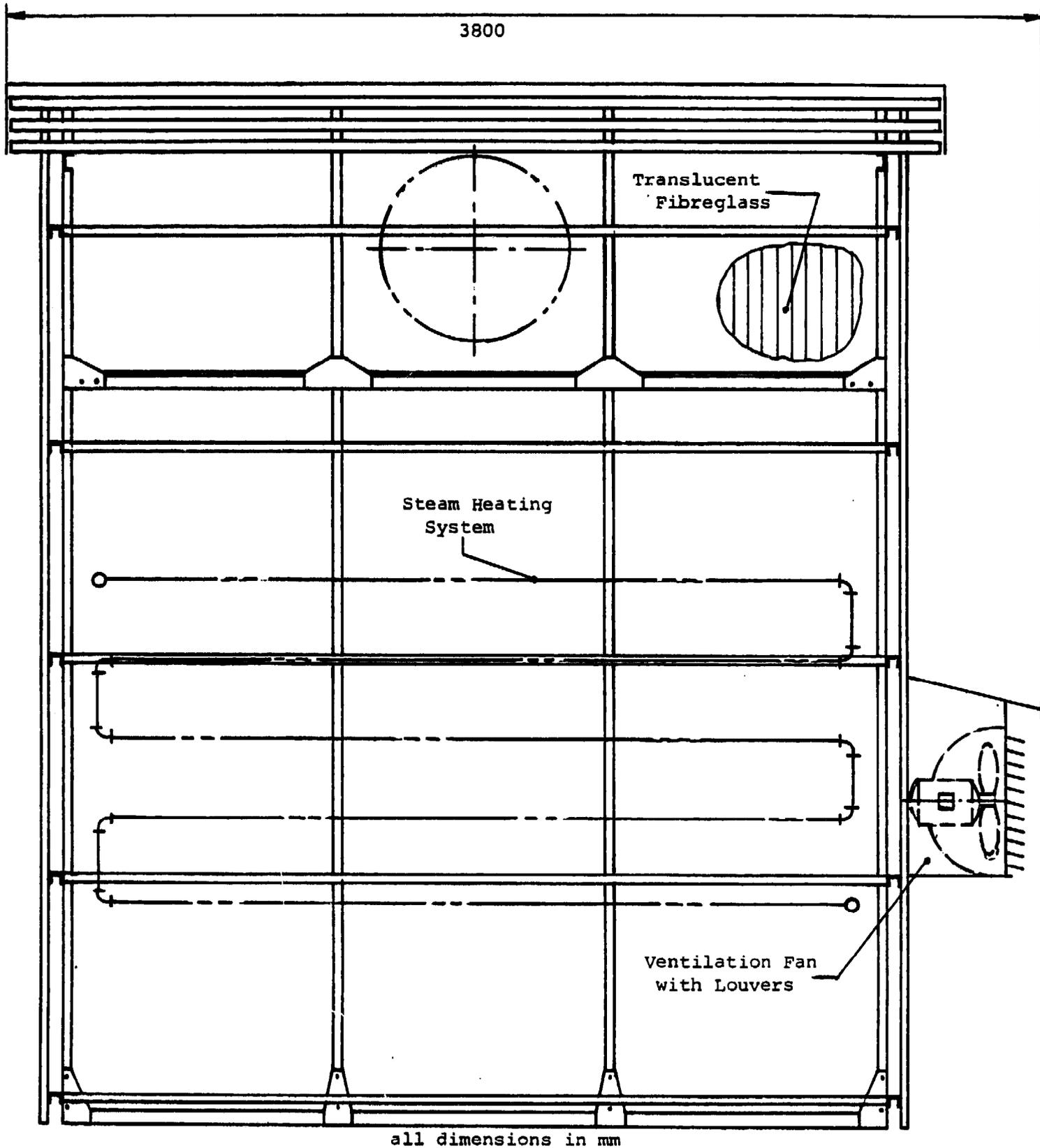
Figure 3. Schematic Plan of the Dryer, Side View
