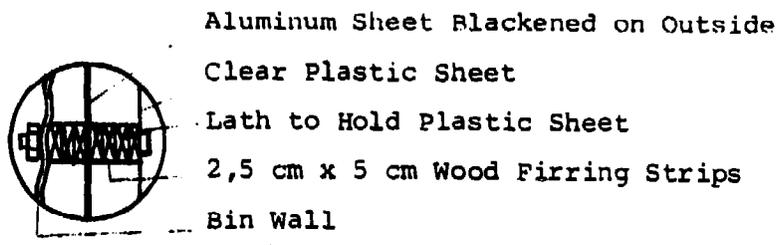
Solar Heater Cross Section
