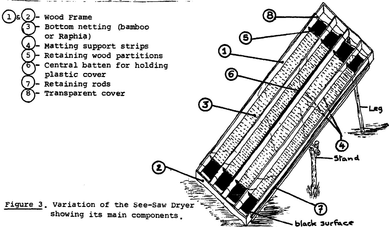
Figure 3. Variation of the See-Saw Dryer showing its main components.
