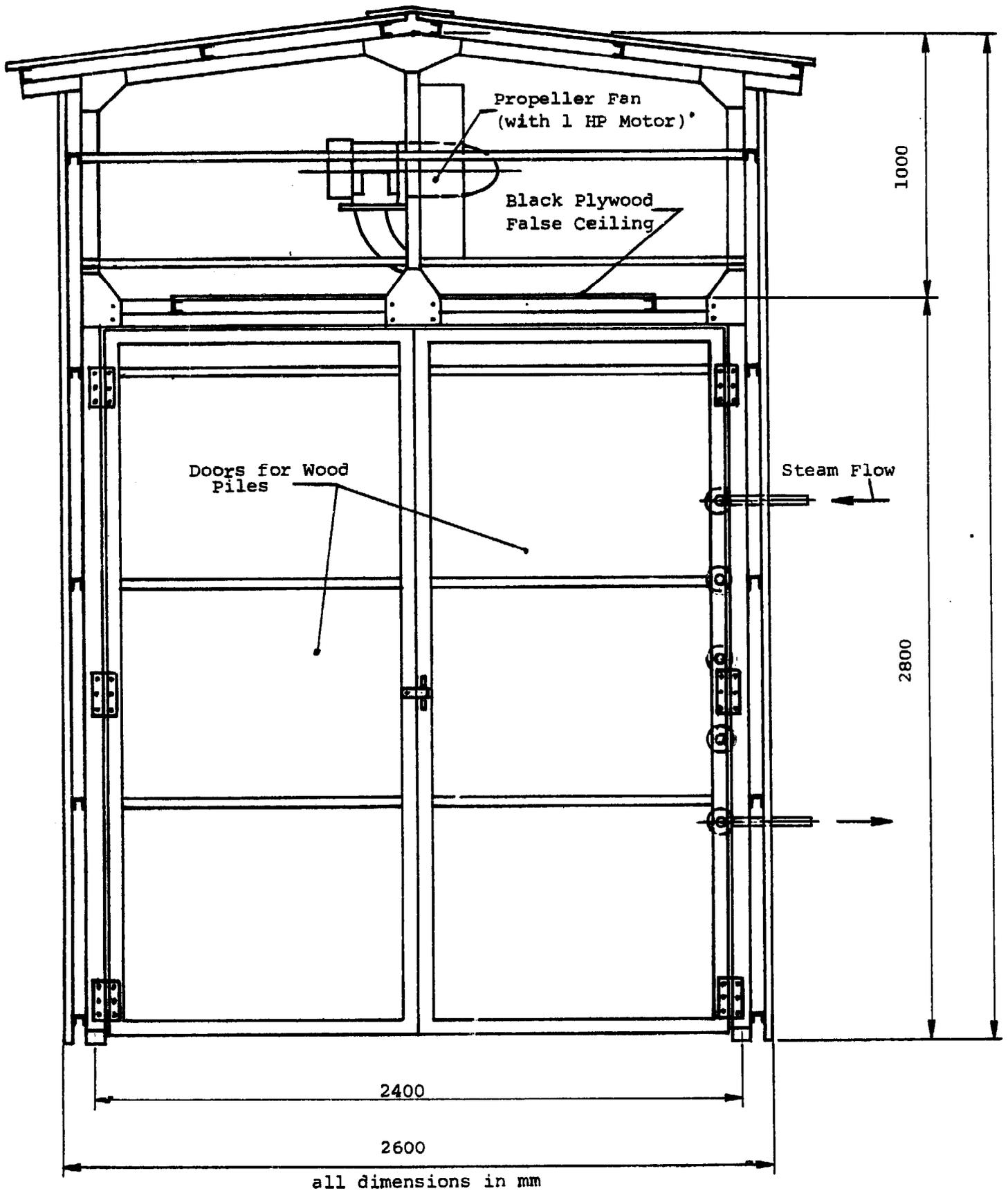
Figure 2. Schematic Plan of the Dryer, Front View
