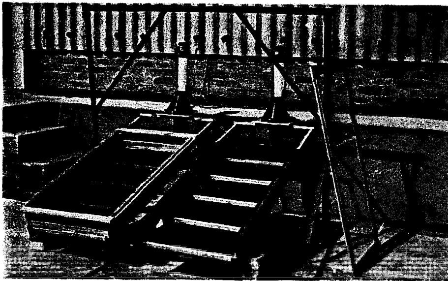
Figure 1. This Picture shows the Experimental Set-Up. On the Left, the Downdraught Dryer and on the Right, the Crossdraught Dryer.
