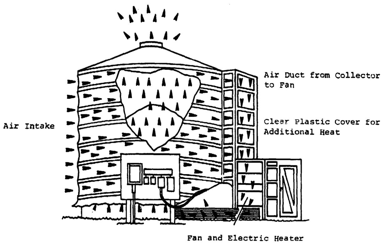
Figure 3. Solar Crop Drying Showing Basic Construction
