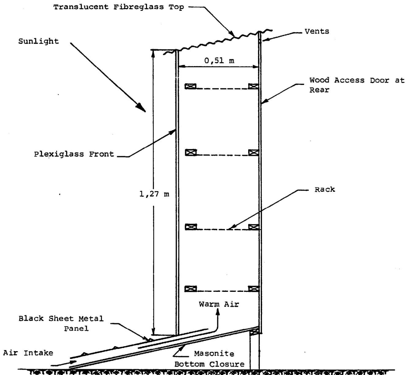
Figure 1. Section View of the Fruit and Vegetable Dryer
