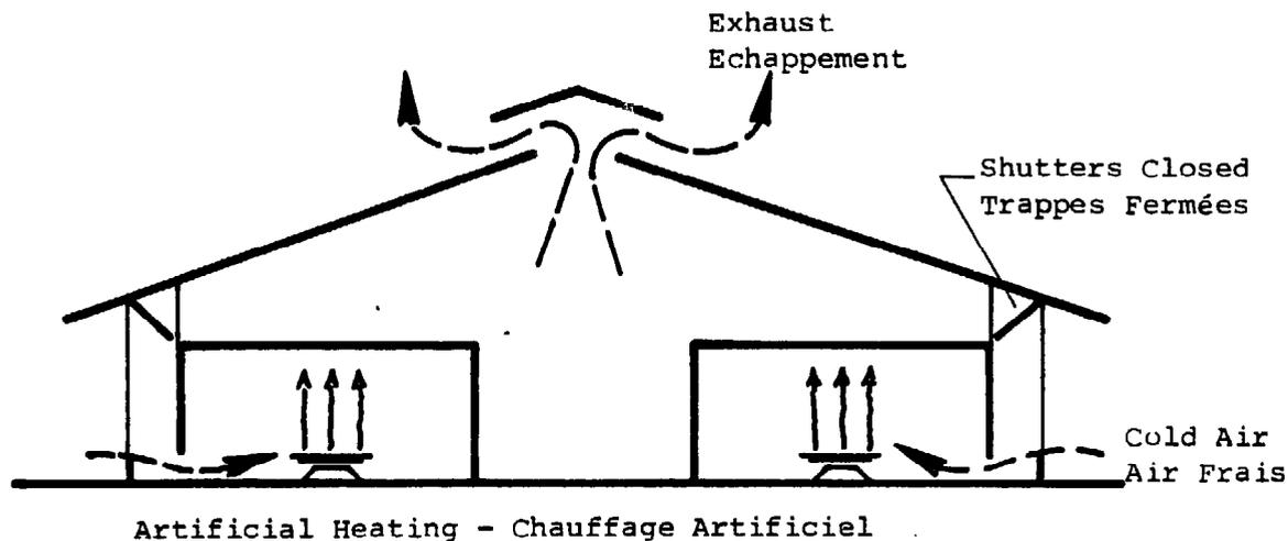
Figure 3. Air Circulation in the Glass-Roof Dryer for its Two Heating Modes
