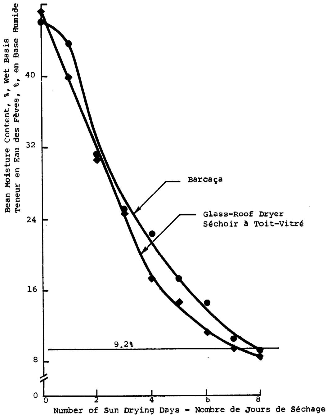
Figure 4. Drying Rate of Cocoa Beans with Solar Energy
