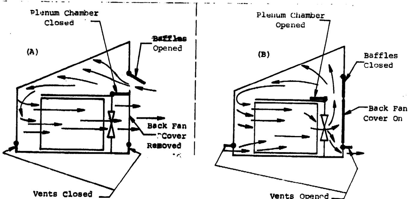
**Figure 3.** Drawing Showing the Kiln Working as (A)
