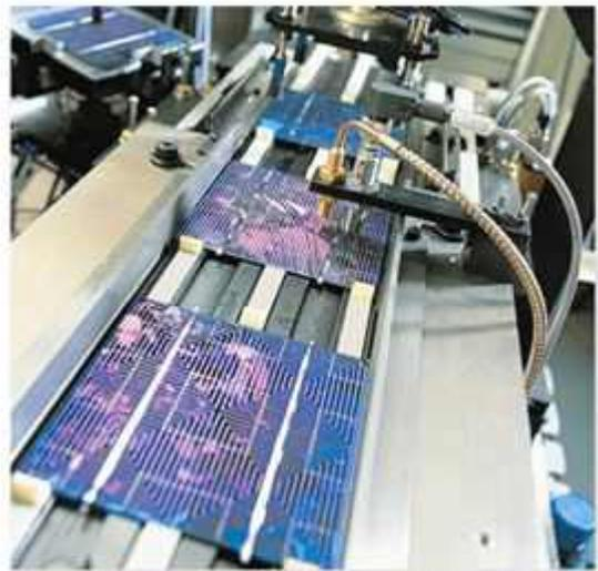
*Printing of Photowatt's front-side PV cells.*
