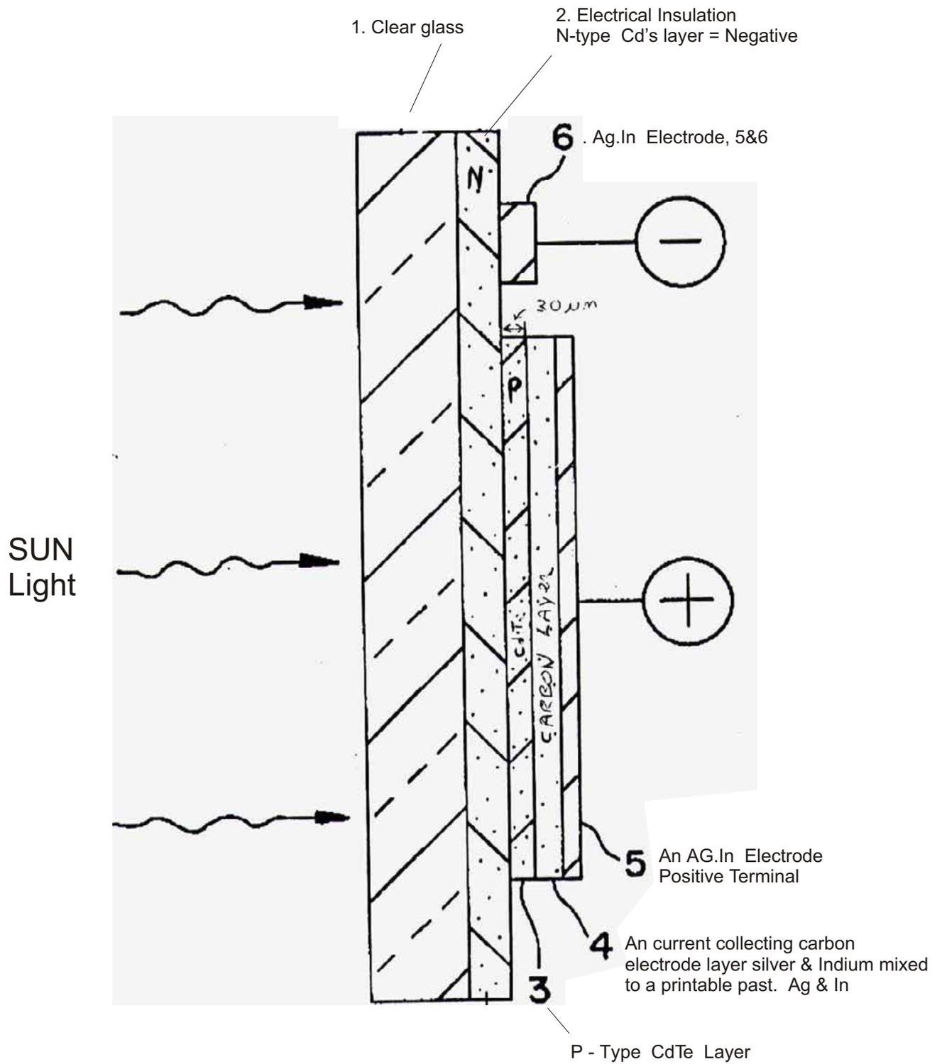
Double or triple print #2, to do this you print the first layer, let dry and then print the 2nd layer = 60 um thickness. #3 layer print only one layer using the same screen printing screen.
