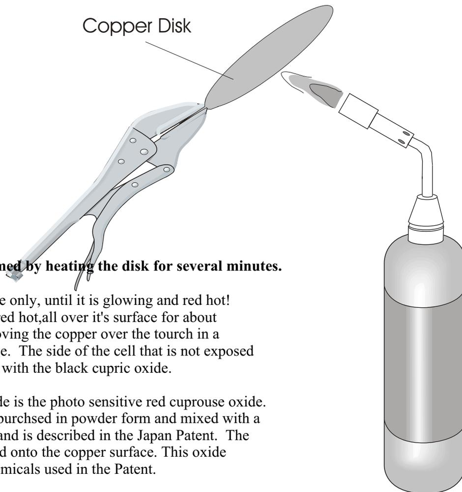
**Photo sensitive oxides are formed by heating the disk for several minutes.**
