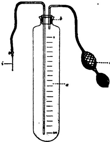
Fig. 66.—Apparatus for the injection of considerable quantities of toxin into the horse: *a*, Graduated cylinder closed by a rubber cork, *b*. Air is pumped into the constant pressure bulb *c*, and from this passes into the cylinder. The toxin is forced out through the needle at *i* (Levaditi).
