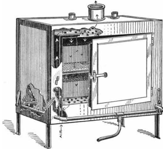
Fig. 48.—Oven for sterilization by hot air (Jordan).
